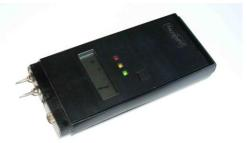
**THE RANGE** of the digital read-out is from 8% to well above fibre saturation (28%) moisture content in wood. Readings above 28% indicate increasing levels of high moisture, but they are **not** percent moisture content.
