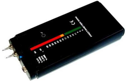
**THE RANGE** marked on the fascia is from 6% moisture content in wood to well above wood fibre saturation point (28%). Readings above 28% indicate increasing levels of high moisture, but they are *not* percent moisture content, they are very approximate. Readings below 10% may be outside the normal percentage error of  $\pm 1\%$  and should not be relied upon. If accuracy in this region is required, then Protimeter's more accurate Timbermaster moisture meter should be used.
