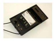
is the standard measurement method in Europe. The Protimeter Timbermaster may also be used for surveying, but note that the accurate sawn and planed wood values given on the 184T are not maintained accurately on chipboard, mdf, plaster or masonry. Such readings are typically very wide of the mark.
