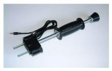
insulated shafts so that the moisture measurement is made between the tips of the needles. This makes it possible to measure moisture content at different depths up to the length of the needles and to obtain readings within the wood which are independent of surface moisture. The hammer probe is fitted with a 3.5mm jack plug and will fit all modern Protimeter instruments.
