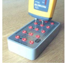
If using the VERUS Checkbox to check the hammer is operational use the 14% value, where probes go diagonally between the two sockets as shown right. To check 27% value, probes go between lower sockets. At each reading observe the display for several seconds to detect any change. 'Rock-steady' readings are obtained if the meter, lead and hammer probe are operating correctly. The hammer probe should give identical readings to the hand probe; if this is not the case investigate further.
