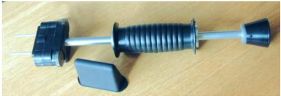
To insert the pins into the measured timber, use both hands and strike until they are deep enough for the reading, up to a maximum of around 1/3 the total depth of the timber. Take care to hammer in and out perfectly straight (dense specimens may not permit desired depth being entered). Readings may be taken as the probe is entered to establish the moisture gradient, unless the timber is kiln dried or old a moisture gradient increasing towards the centre is expected.
