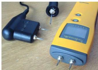
When used with the optional temperature probe (illustrated centre), the moisture measurements are automatically corrected with respect to temperature. This last feature is particularly relevant for users measuring wood that is significantly above or below 20°C.
