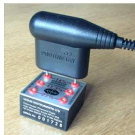
placing the electrode needles into the sockets of the Verus Checkbox (traceable if in recent calibration) accessory). The optional VERUS Checkbox Model II illustrated top, checks a meter at 3 moisture scale points. When checking the calibration, the Timbermaster A-scale (European redwood) should be selected and the temperature probe must be disconnected. Correctly set a Timbermaster will register within 0.3% emc of the marked Verus Checkbox facia value.
